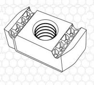
Channel Nuts are self centering and are manufactured from quality steel with zinc plated finish to BS 3382 Part 2 For best results use M 12 size. Recommended tightened tension is 5-7 Kgf.
