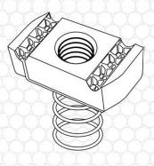
Channel Nuts are self centering and are manufactured from quality steel with zinc plated finish to BS 3382 Part 2 For best results use M 12 size. Recommended tightened tension is 5-7 Kgf.
