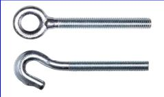
JCP Hook and Eye Bolts are forged hooks and eyes with a metric thread and are zinc plated and clear passivated to a min 5µm.
