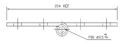
Mild Steel to BS1449 Section 1.2 KHR4P or Q195 max. Carbon 0.08% **Materials:**
