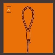
Loop end to form a choke knot for wrap around anchor points, purlins or I-beams.
