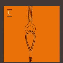
M8x60 eyebolt used in conjunction with female threaded components. Ensure components are compatible to complete the installation.
